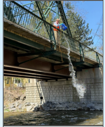
Fall Creek volunteer, Charlie Trautmann, collects water samples using a bucket, as limited shoreline access at this site requires an alternative sampling approach to safely reach the stream.
