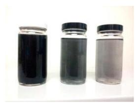
Rubber may be breaking down in your plumbing gaskets, or carbon pieces are leaking out of your household water filters. Replace both as needed. You may have iron or manganese adding color from old corroded pipes. Contact the Water Quality Line and ask for a water test kit that includes testing for iron and manganese. Iron is not a health risk, but higher levels of manganese may pose a health risk.
