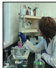
Chemical Analyst Casey Halton tests samples for chloride, an indicator for brine waste
