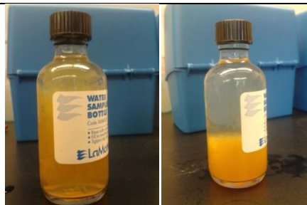
Step 4 - Wait until the precipitate has settled below the shoulder (shown on right) before adding the sulfuric acid
