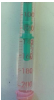
In this picture, the result is 136 mg/L.
