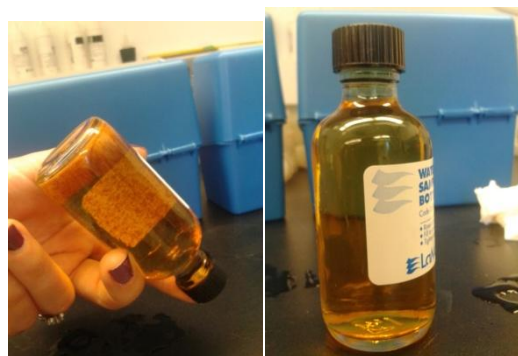
Step 6 - Invert the bottle until the precipitate has fully dissolved before adding to test tube.
