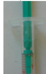
Step 4 - Fill titrator so that the green ring is at the 0 line (shown)
